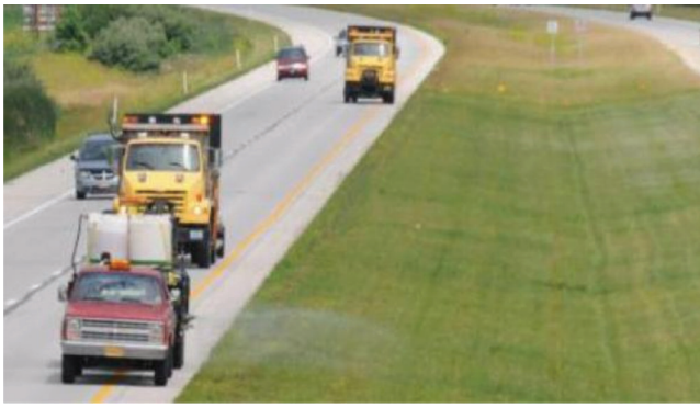
Figure 2.2 Photograph of research skid sprayer holding six 100-gallon herbicide tanks.
