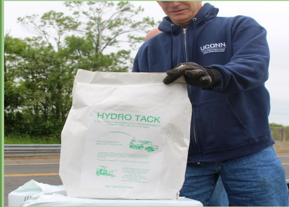
Tackifier used to bind mulch to the soil.
