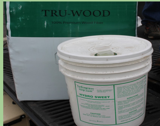
Wood fiber mulch and Hydro Sweet, used to neutralize acid soil conditions.
