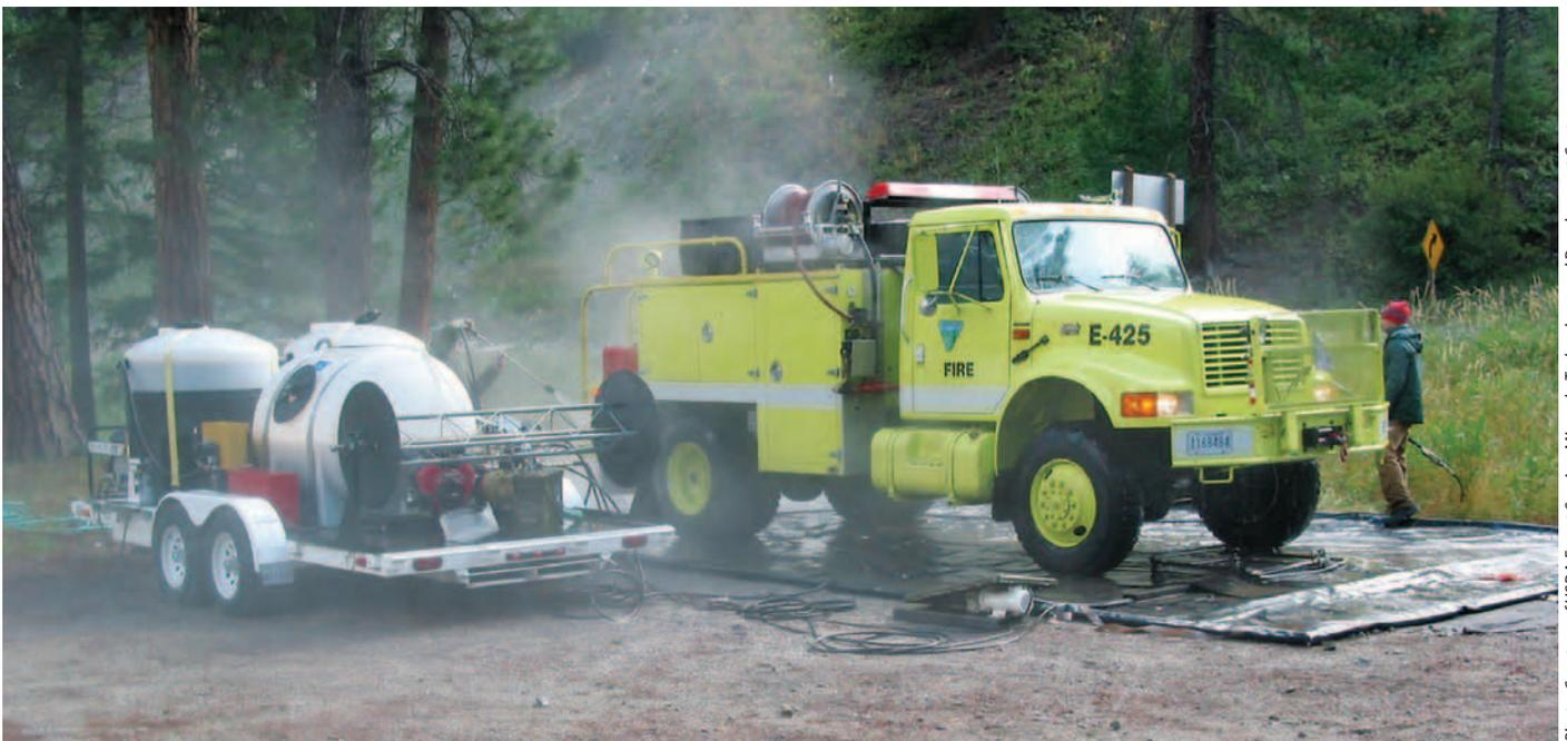
*The Forest Service designed this portable washer to clean vehicles in challenging terrain. The system fits on a trailer and can be towed by a pickup truck. It reuses wash water and is inexpensive.*
