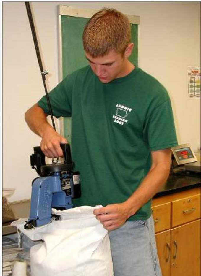
Student employee bags seed using Fischbein portable bag sewing machine.
